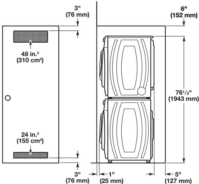
\* Add spacing of 1" (25 mm) on all sides of washer/dryer.
