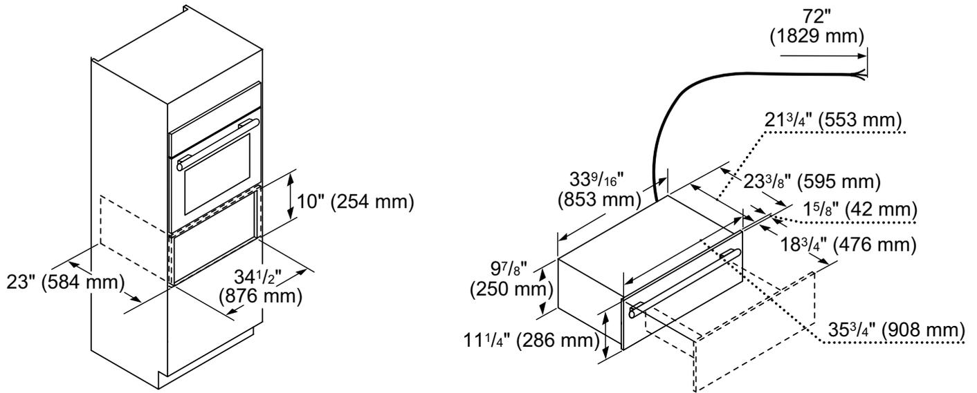
**NOTE:** 1 5/8" is the depth of the standard front panel (includes gasket). Dimension is not valid for custom panel product.
