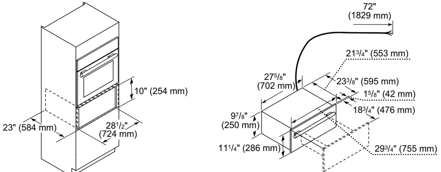
**NOTE:** 1 5/8" is the depth of the standard front panel (includes gasket). Dimension is not valid for custom panel product.
